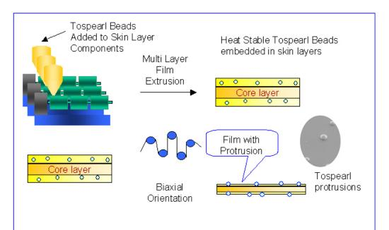
Heat stable Tospearl beads can be added to the skin layers of BOPP films by a multi-layer extrusion process. After biaxial orientation by stretching, the beads protrude from the surface of the films and act as anti-blocking agents.
