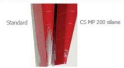
CoatOSil MP 200 silane can help improve bending resistance of 2K HS epoxy primer. It can minimize impact of accelerating catalyst on bending resistance.
