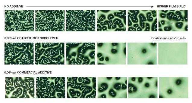
Additionally, these clearcoat samples were applied directly over the glass substrate to evaluate flow and leveling over a distinctly different substrate.
