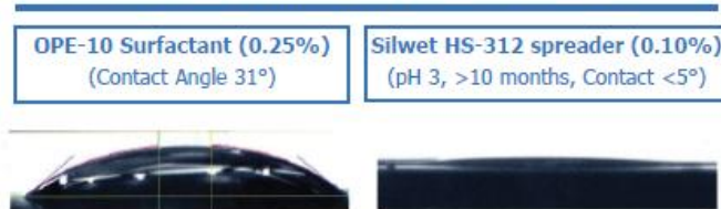
Figure 1: Contact Angles of Spreader Adjuvants
