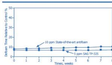
Figure 2: Relative Defoam Time of Antifoams as Measured in Wet High-Foaming Neat Diesel Fuel
