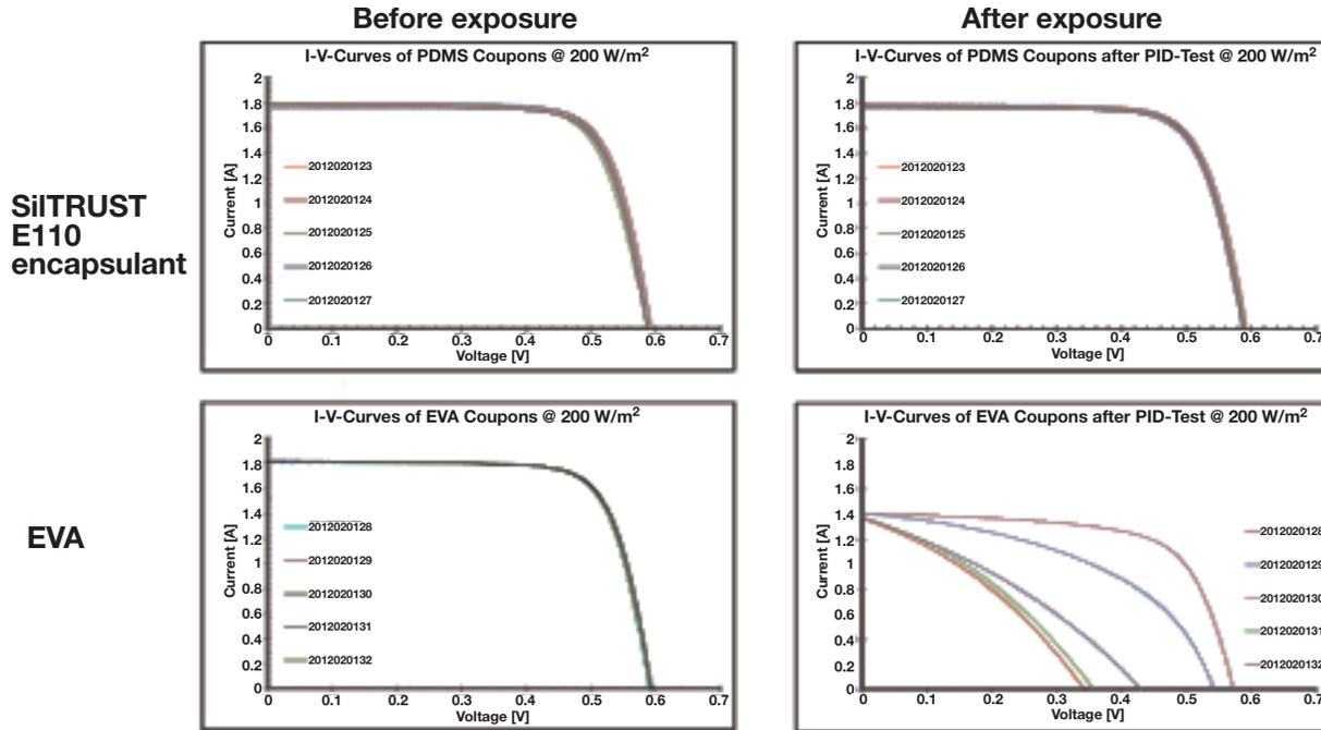
I-V-curves before and after 48 hours @ 85 °C/85%RH with -600V (single cells) @ 200 W/m<sup>2</sup> irradiation.
