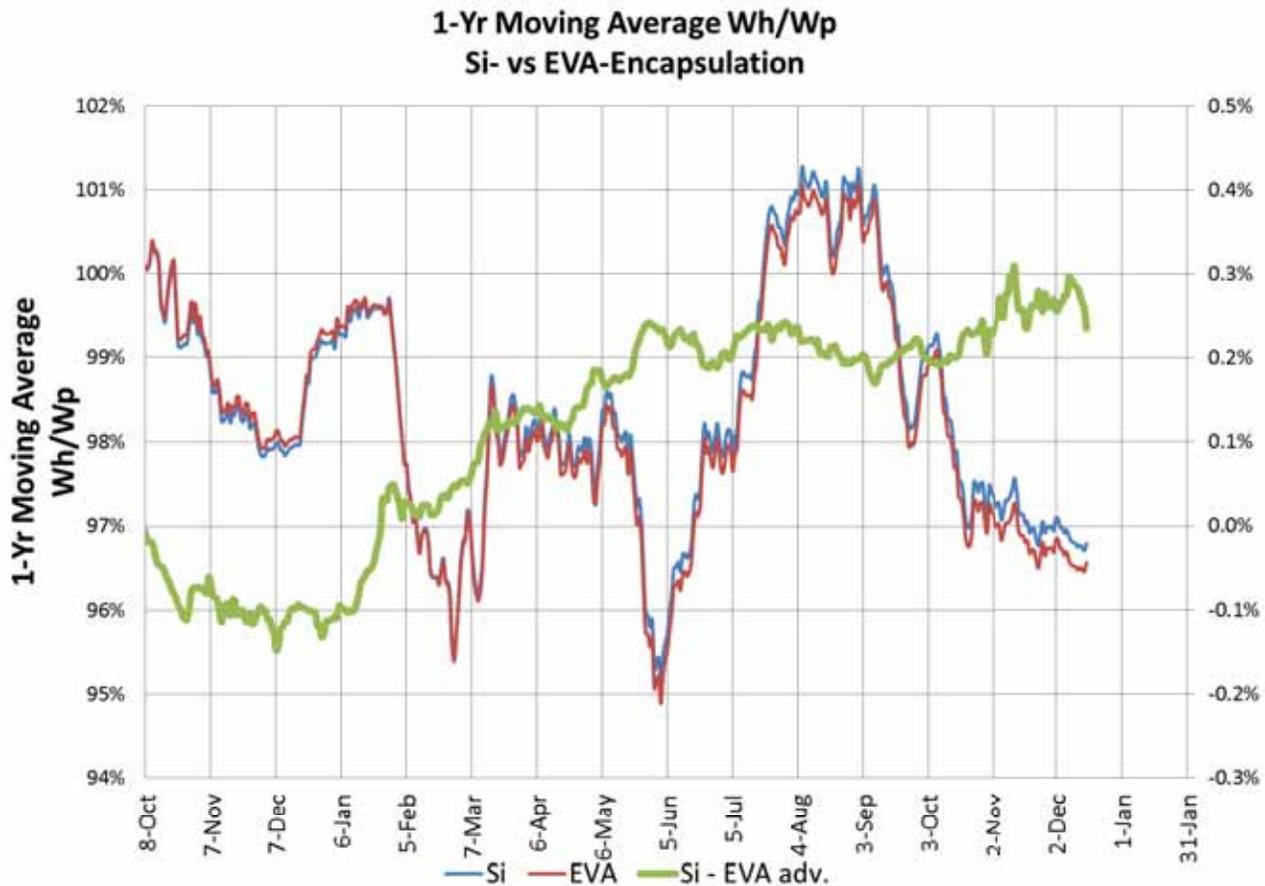
Increasing efficiency benefit over time is shown after two years of outdoor operation. Plotted are the 365-day moving averages of Wh/Wp for EVA-encapsulated modules (red line) and the SiTRUST E110 encapsulated modules (blue line), as well as the increasing relative difference between them (green line).
