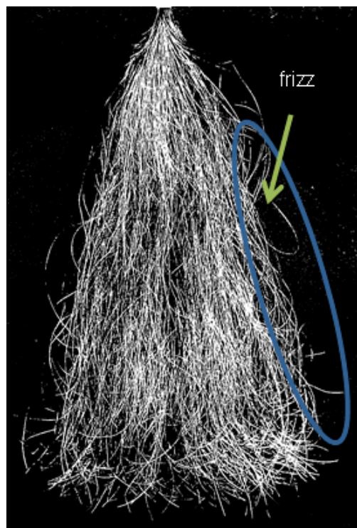
Figure 7: Binarized Image of the Hair Tress for Curl and Frizz Reduction Assessment
