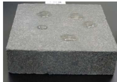
Figure 2: Slight Beading Effect of Silblock WMS Masonry Water Repellent Treated Concrete
