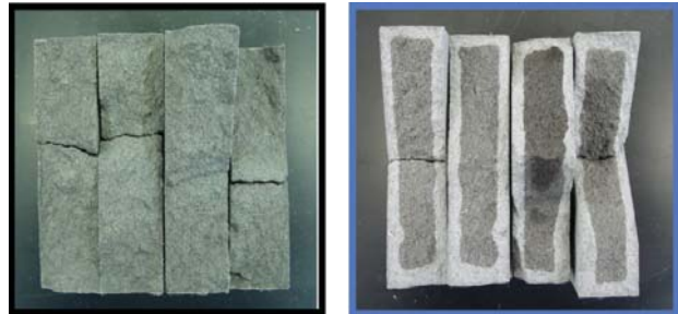
Figure 1: India Ink Penetration Depths with Silblock WMS Masonry Water Repellent (right) as Compared to Control (left)
