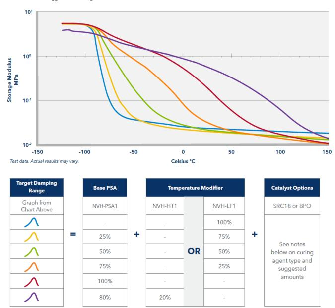
The catalyst options, SRC18 or BPO, drive crosslinking. As a rule of thumb, the more catalyst used, the lower the peak damping properties will be. It is suggested to use as little catalyst as necessary to achieve good cure. This will help maximize damping performance.
