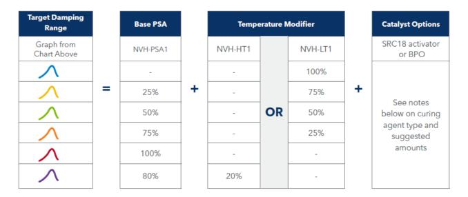
The catalyst options for driving crosslinking include Momentive SRC18 cure activator and BPO. As a rule of thumb, the more catalyst used, the lower the peak damping properties will be. Therefore, use of the minimum amount of catalyst necessary to achieve good cure is recommended in order to help maximize damping performance.
