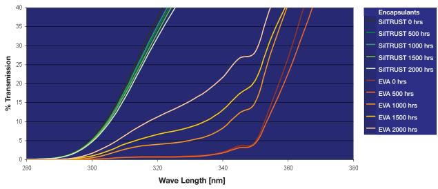
UV-VIS Spectral Changes Upon Damp Heat (85 °C / 85%RH) Aging (Glass-Encap-Glass Assembly)
