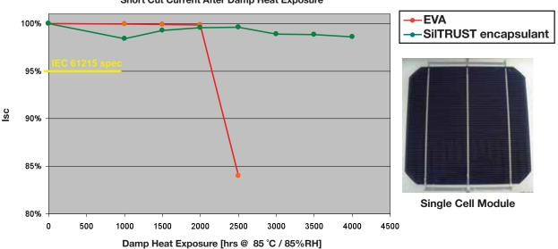
Short Cut Current After Damp Heat Exposure
