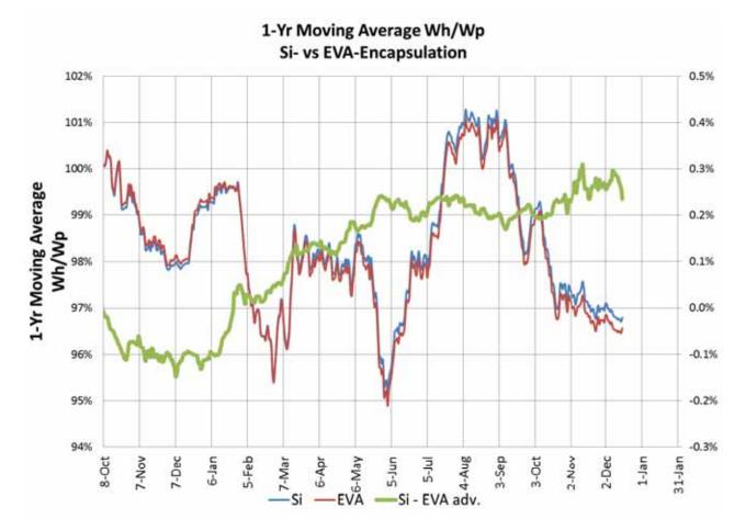
Increasing efficiency benefit over time is shown after two years of outdoor operation. Plotted are the 365-day moving averages of Wh/Wp for EVA-encapsulated modules (red line) and the SiITRUST E110 encapsulated modules (blue line), as well as the increasing relative difference between them (green line).
