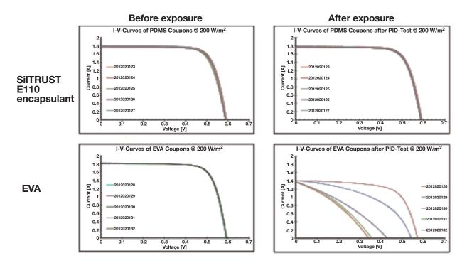
IV-curves before and after 48 hours @ 85 °C/85%RH with -600V (single cells) @ 200 W/m<sup>2</sup> irradiation.
