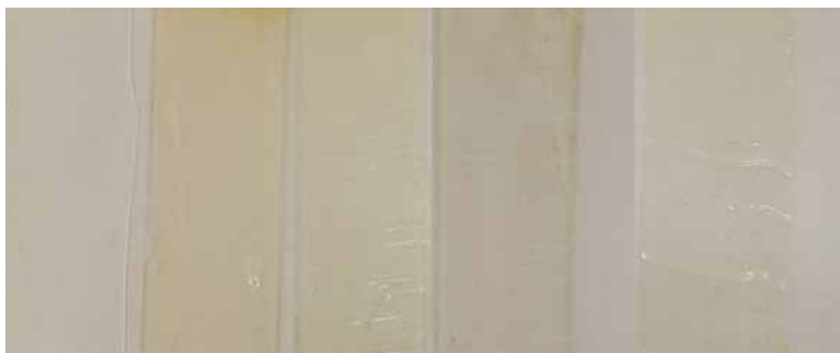
No Aminosilane Silquest A-2120 Silane Silquest A-1110 Silane Competitive Benchmark: Oligomeric Aminosilane Silquest A-Link 600 Silane
