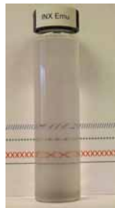
Figure 8 - SilForm INX fluid can be Dispersed to Make a Clear Solution for Ease of Use in an Aqueous Formulation
