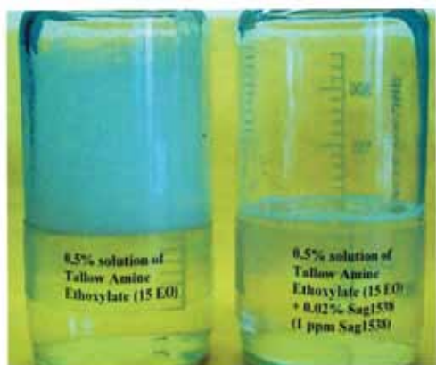
Figure 2: SAG 1538 Silicone Antifoam Defoaming in Tallow Amine Ethoxylate (0.5%)
