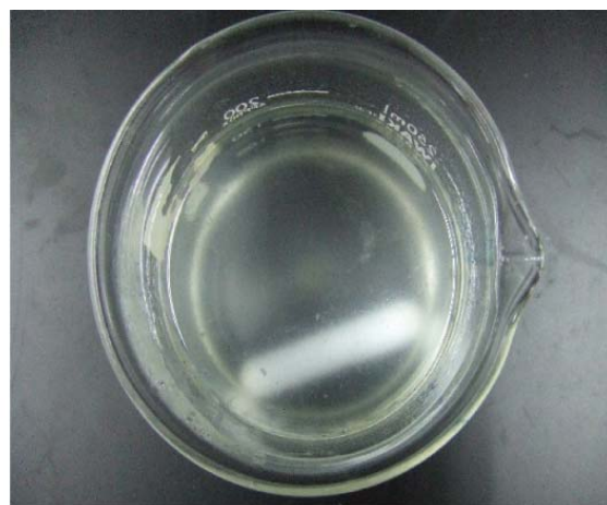
Top view of Amino emulsion at pH 7 at 70°C 1% actives dispersion in water Hazy, oiling observed
