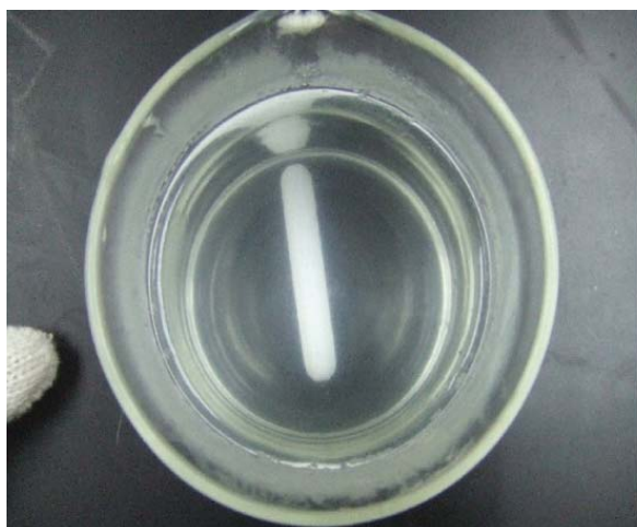
Top View of Magnasoft 238 textile enhancer at pH 7 at 70°C 1% actives dispersion in water Clear, no oiling observed
