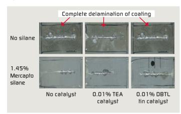
Figure 2: Corrosion resistance on galvanised metals, showing improvement due to silane addition.
