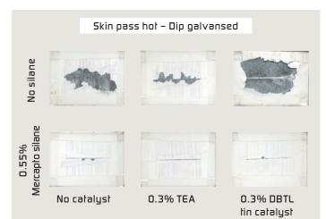
for one week at ambient conditions. The corrosion resistance of the cured panels was tested in neutral salt spray for 500 hours. Coatings without silane delaminated completely while the coatings using the silane did not show any delamination (*Figure 7*).
