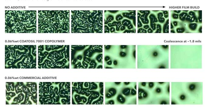
Additionally, these clearcoat samples were applied directly over the glass substrate to evaluate flow and leveling over a distinctly different substrate.
