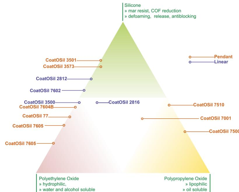
The effect of silicone additives on a coating strongly depends on their mutual compatibility. Compatibility is controlled by the amount of polyethylene oxide (EO), polypropylene oxide (PO), and polydimethylsiloxanes (PDMS) in a molecule.
