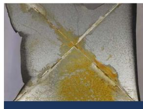
2K WB Epoxy MIO primer control coating w/o silane adhesion promoter. After 240h of NSST exposure of CRS panel coated with the epoxy primer coating film delaminates from the metal substrate.
