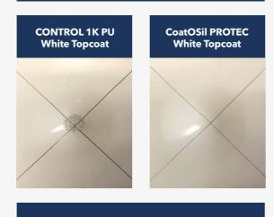
Impact resistance and cross-section adhesion after 2h immersion in boiling water. Excellent film integrity, flexibility and wet adhesion with CoatOSil PROTEC technology.
