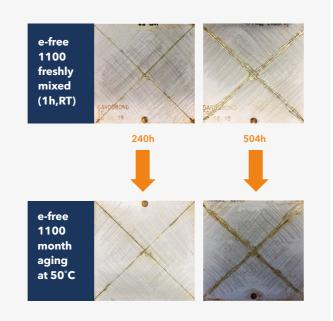
2K WB low bake Epoxy MIO primer control coating with e free 1100 silane solution adhesion promoter on CRS . Test panels with e-free 1100 silane demonstrated improved corrosion resistance after 240 and 504 hrs neutral salt spray testing for both fresh and heat-aged formulations.
