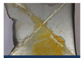
2K WB Epoxy MIO primer control coating w/o silane adhesion promoter. After 240h of NSST exposure of CRS panel coated with the epoxy primer coating film delaminates from the metal substrate.
