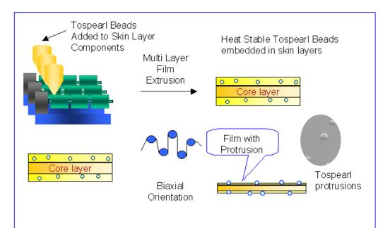
Heat stable Tospearl beads can be added to the skin layers of BOPP films by a multi-layer extrusion process. After biaxial orientation by stretching, the beads protrude from the surface of the films and act as anti-blocking agents.
