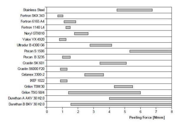
Left end of bar are values "As moulded"; right end of the bar after "100°C / 1 h".
