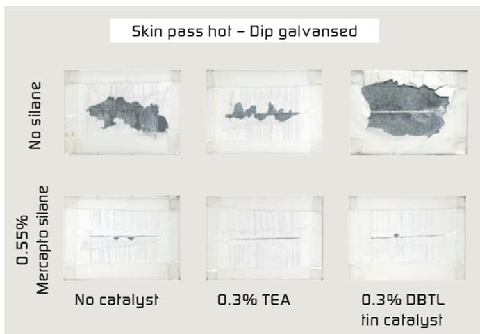
for one week at ambient conditions. The corrosion resistance of the cured panels was tested in neutral salt spray for 500 hours. Coatings without silane delaminated completely while the coatings using the silane did not show any delamination (Figure 7).
