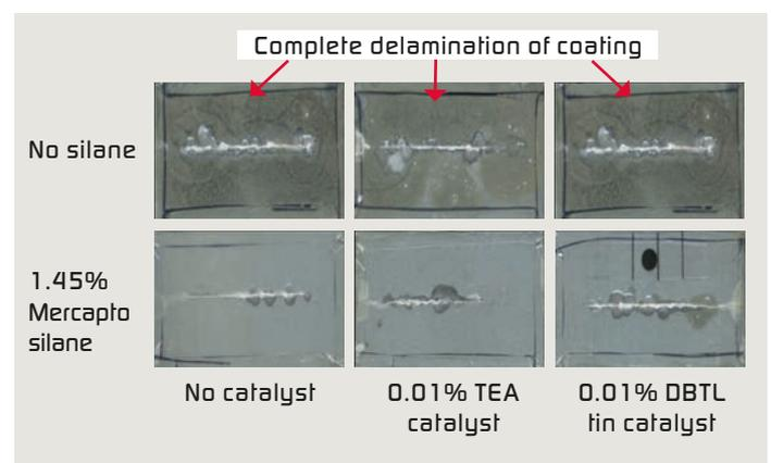
Figure 3: Adhesion test results; control vs. silane addition.
